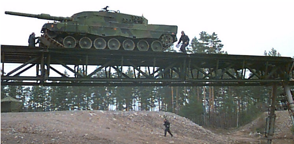
Fig. 12. Fast bridge used as a continuous bridge loaded by a tank.
